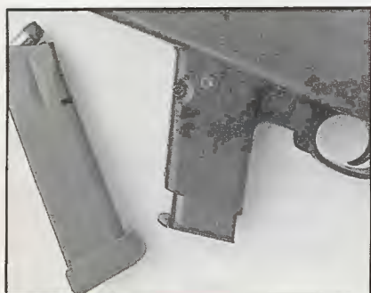
K.C. Enterprises modified this Marlin Camp .45 to accept Para-Ordnance P14.45 13-round magazines.
